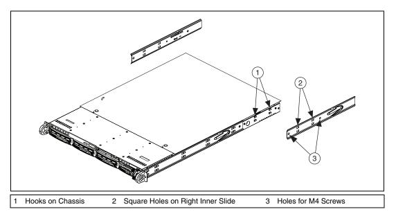
Figure 2-1. Installing Inner Slides
